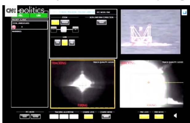
Here's one of the consoles they look at. They 1) see the target in one of the screens, 2) they put the dot on the part they want to "take out," and then, 3) push the button. In both the lower middle, and the lower right screens, you see the target exploding in a ball of flame. Since the laser is invisible, [unless it travels through smoke] no one sees it, hears it, or knows anything except that the target just exploded in flame. How did it happen? And why? No one knows - except those who know.
