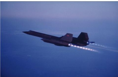
At 2,200 mph, it's traveling 200 feet per second faster than a high-speed bullet. The friction super-heats the titanium skin to 1000 degrees - which is hot enough to melt lead.
